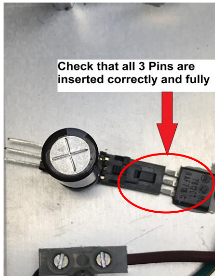
Figure 4 – Capacitor Assembly (C015A) to 7812
